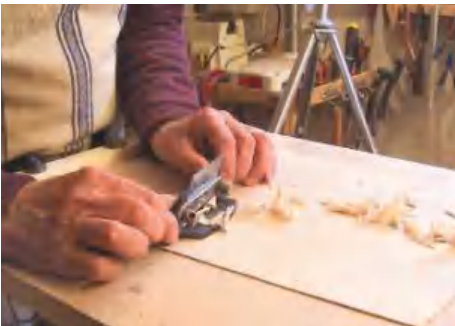
▲ Pic.10 The No.080 cabinet scraper in use
